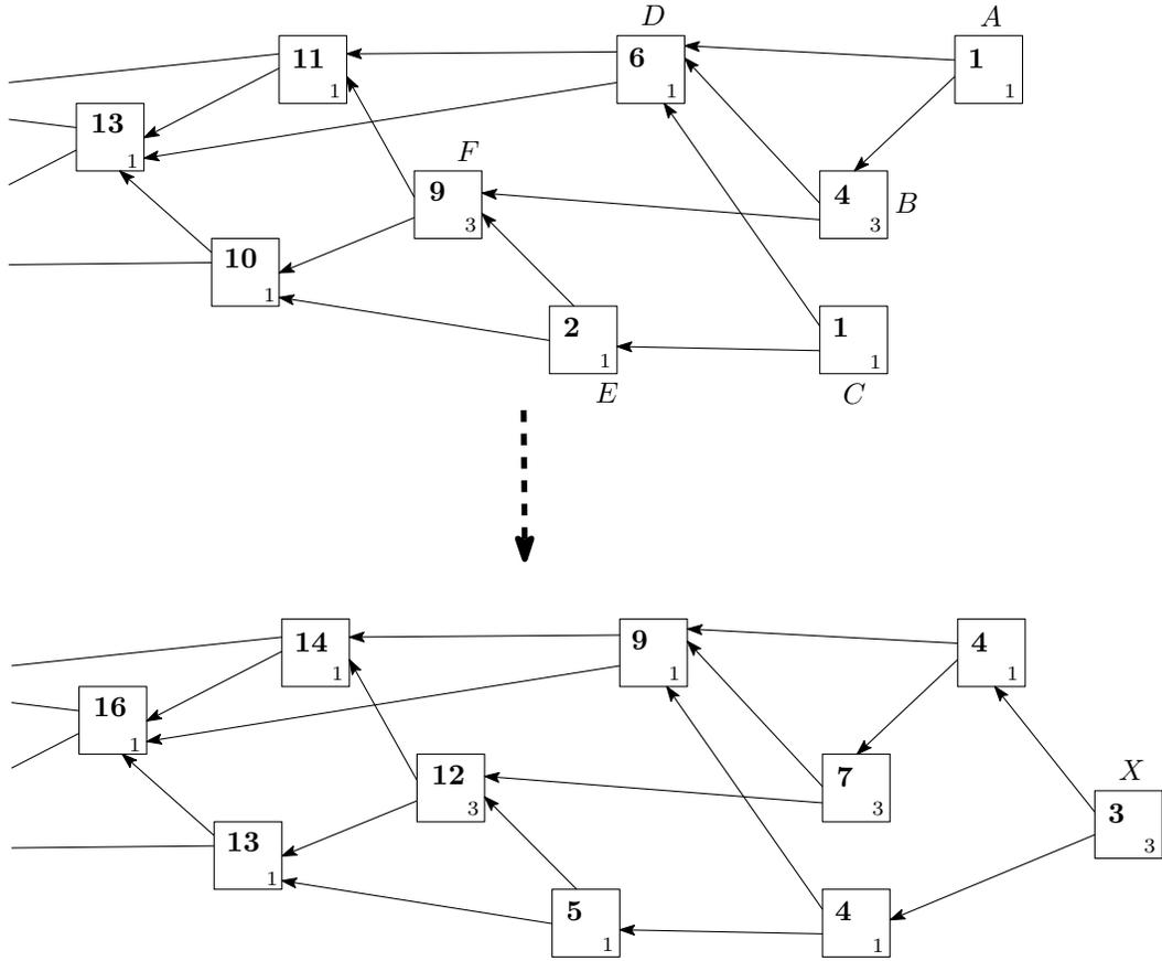
Figure 1: DAG with weight assignments before and after a newly issued transaction,  $X$ . The boxes represent transactions, the small number in the SE corner of each box denotes own weight, and the bold number denotes the cumulative weight.
